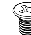
Vis à tête fraisée M5*8 (6pcs = 4pcs + 2pcs de remplacement) M5 x 8 Countersunk head screw (6pcs = 4pcs + 2pcs replacement)
